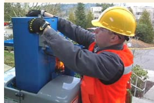
The covered steel telescoping mast is built for durability in rough work environments.
