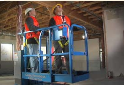
A standard extension deck holds two workers with up to 1 sq m (1,550 sq in) of workspace.
