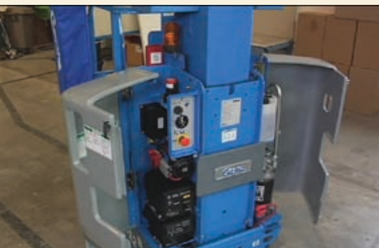
Durable, flexible ABS material helps the rear access covers maintain their shape. They open wide for easy service access.
