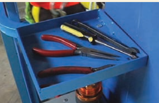
Standard work trays on both sides of the mast keep tools and fasteners handy.
